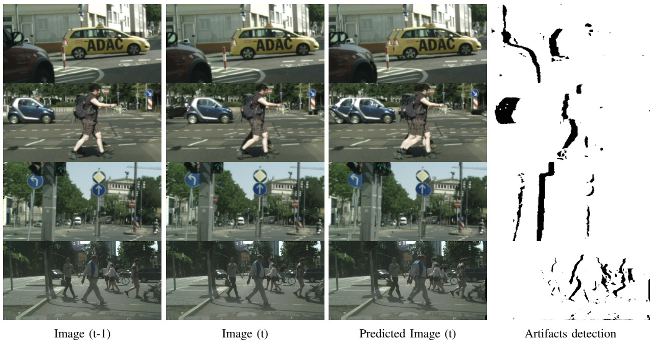
Fig. 3: Examples of artifacts detection with direct optical flow in Cityscapes data set
